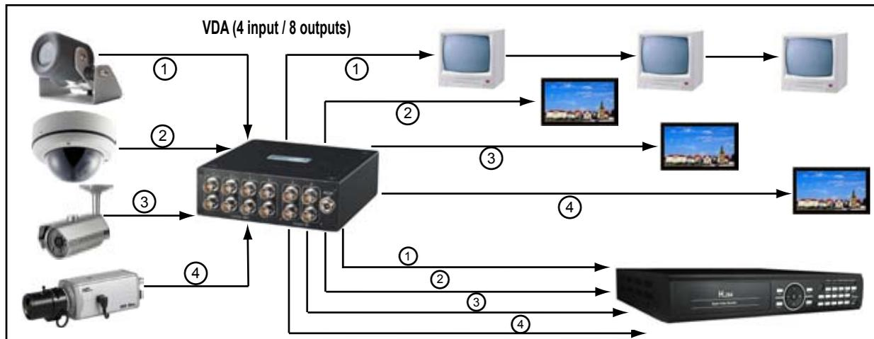
Diagram 3: Example of 4 Input / 8 Output Video Distribution Amplifier Set-Up
