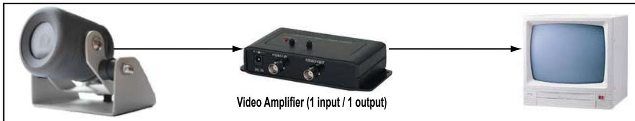
Diagram 1: Example of Video Amplifier Installed to Boost Signal to Remote Monitor
