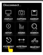
On CMS program, a user can remotely operate PTZ cameras and the function includes ZOOM, FOCUS, PRESET, TOURING.
