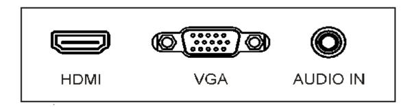
VGA INPUT: D-SUB 15 pins Connector
