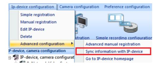
4) Or Select directly "Sync information with IP-Device" at the Advaced configuration from Ip-device configuration menu on on the left side bottom sub part. You need to click on right button of the mouse.
