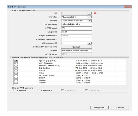
3) Selecting method is same with "IP-device manual registration", and you can edit all information but A (ID). You need to selet resolution supported by IP-device.
