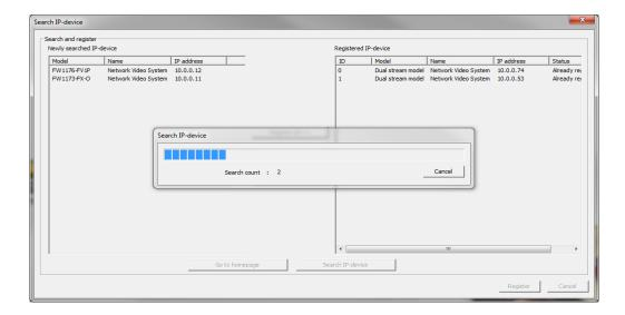
3) **Select** and **move** the cameras that you want to register from the left (Newly searched IP-device) to the right (Registered IP-device) section with the **Register selected** button, and then click **Register**
