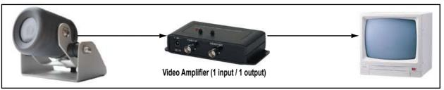
Diagram 1: Example of Video Amplifier Installed to Boost Signal to Remote Monitor
